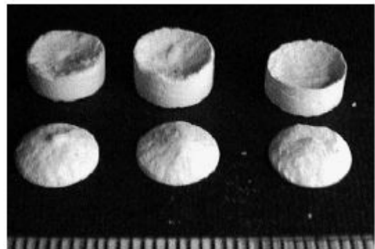
Figure (9) photography of broken tablets upon ejection
